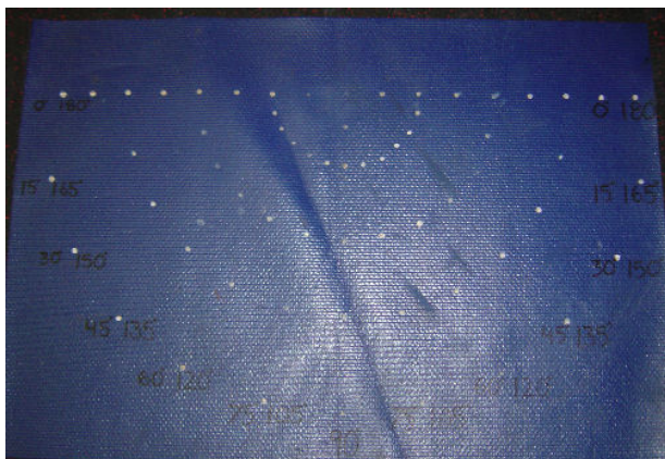
Our “knee mat” to measure arm angle and knee angle
